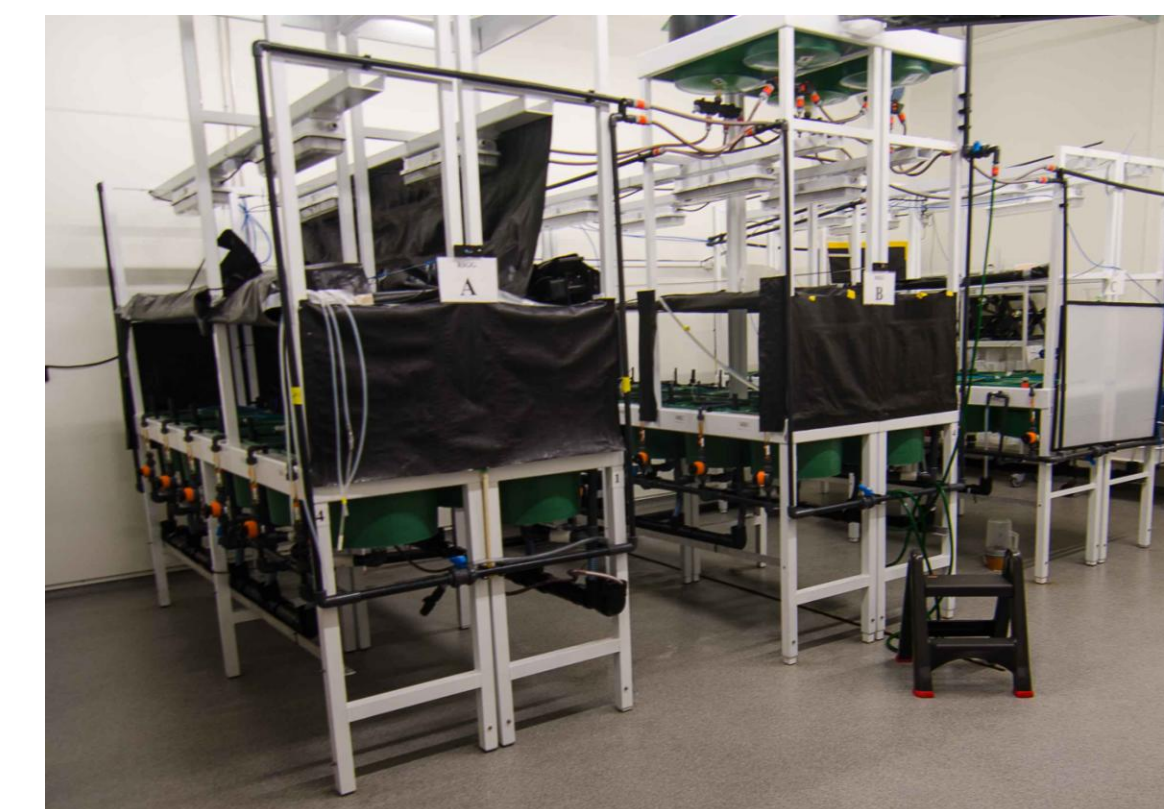
Treatment tanks in cold room Temperature maintained at 12°C
