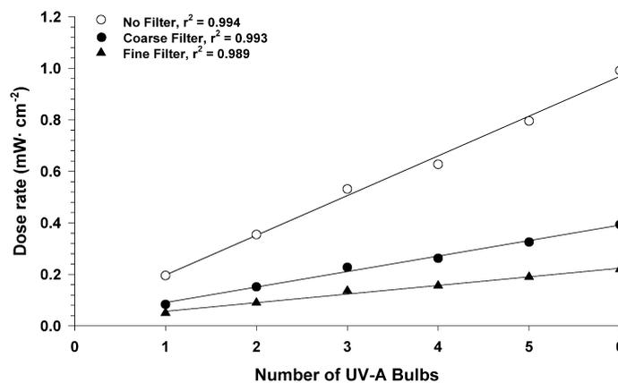
Fig. 2. Sample of different UV-A (320 to 400 nm) dose rates (unweighted) for different numbers of Bachofer bulbs with either no mesh filter, a coarse metal-mesh filter or a fine metal filter. In this example the scaffolding holding the UV-A bulbs was suspended at 33 cm above the phototron.
