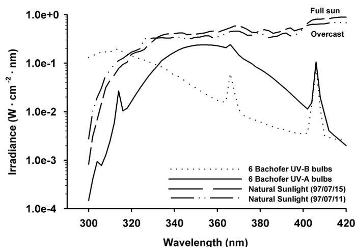
Fig. 1. Irradiance spectra achieved by placing six Bachofer UV-A (peak 365 nm) and UV-B (peak 312 nm) bulbs at 33 cm height above the phototron. Also shown, for comparison, are natural sunlight spectra for a sunny day (97/07/15) and an overcast day measured in Saskatoon, Canada on 97/07/15 and 97/07/11, respectively. Note log scale.
