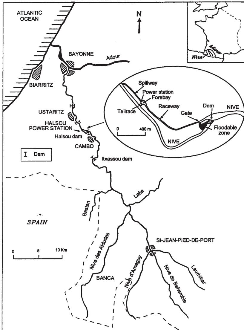
Figure 1. Geographical location and general view of the Halsou hydroelectric plant
