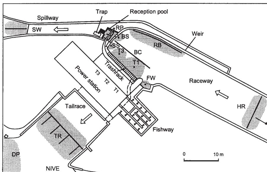
Figure 2. General view of the Halsou hydroelectric power plant and radiotelemetry surveillance zones (see text for explanations)
